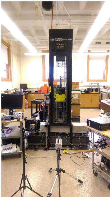
Figure 1.10: Instron dynatup 8250 impact testing machine and set-up
